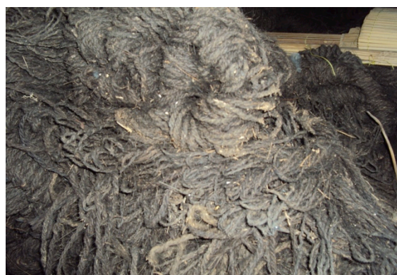
Tying material used to connect bamboo elements in bamboo house construction; also another NTFP derived from the dried leaf sheaths of palms.
