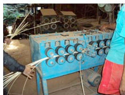
Fig. 5. Rattan treatment facility and rattan derivatizing machine adopted from Vietnam and used by a Cambodian rattan furniture maker.
